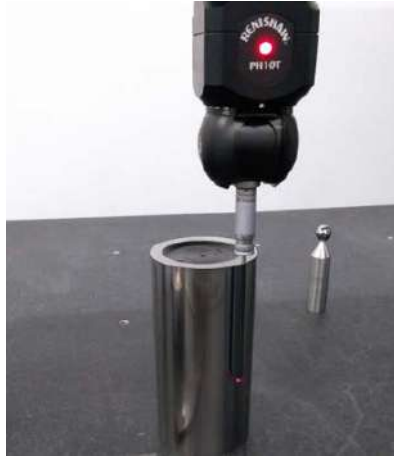
Figure II-7: The cylinder square used for the testing.
