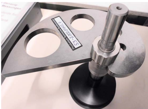
Involute standards: plain profile and with three sinewaves superimposed (freeform)
