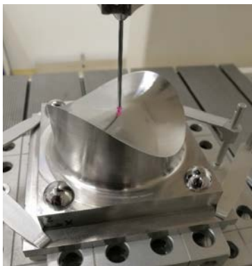
Involute standards: plain profile and with three sinewaves superimposed (freeform)
