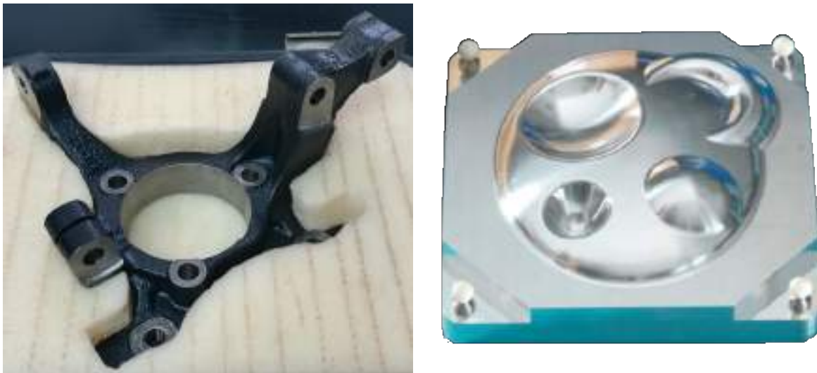
Figure 3-9: The steering knuckle (left) and freeform plate (right) were also selected for the validation study, but adverse conditions prevented them from entering circulation.
