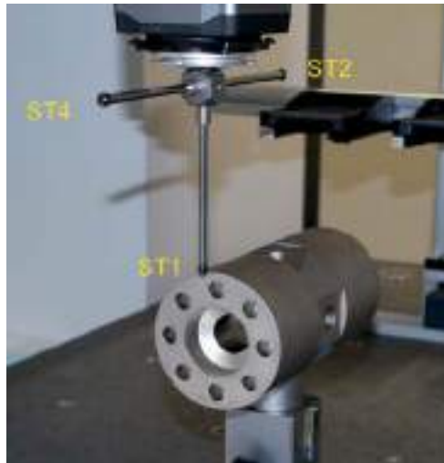
Figure 3-4: A multi-feature check being measured.
